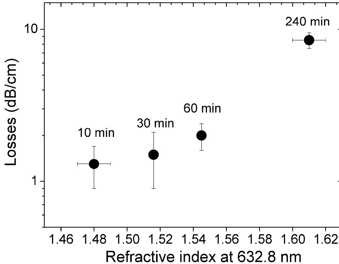
Losses at 1600 nm are essentially propagation losses of the rib loaded waveguide
